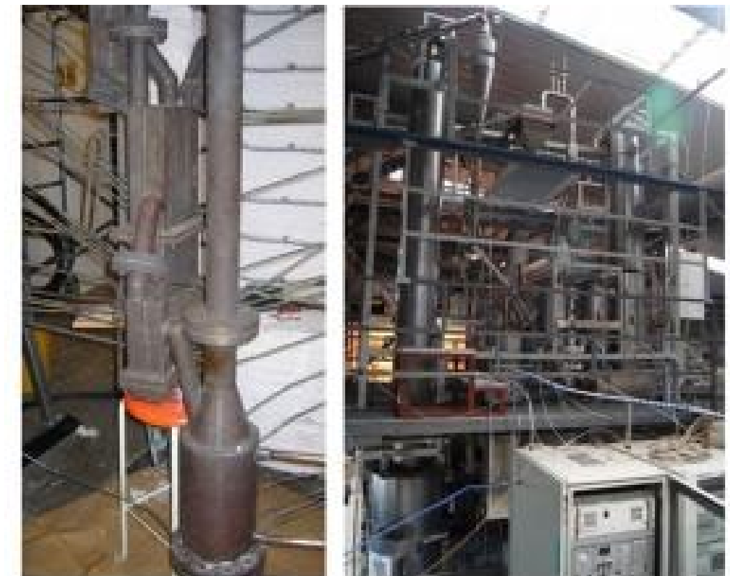
10 kW CLC pilot reactor (left) and 20 kW CLC pilot plant (right)
