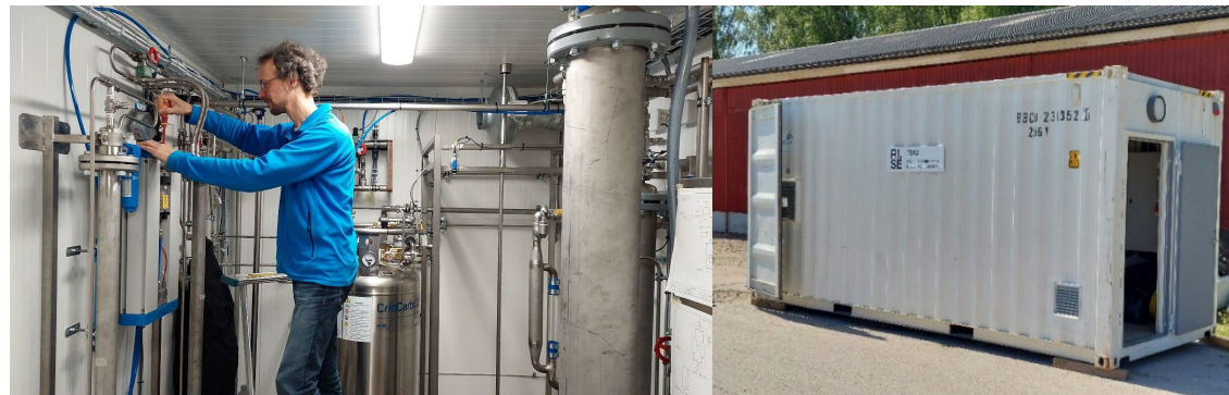
portable gas cleaning pilot plant
