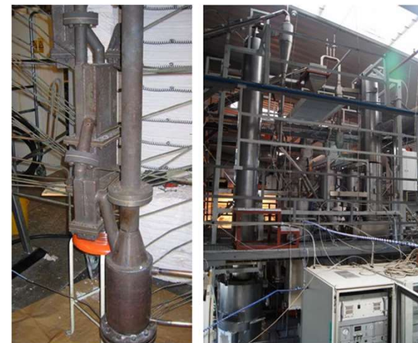
10 kW CLC pilot reactor (left) and 20 kW CLC pilot plant (right)
